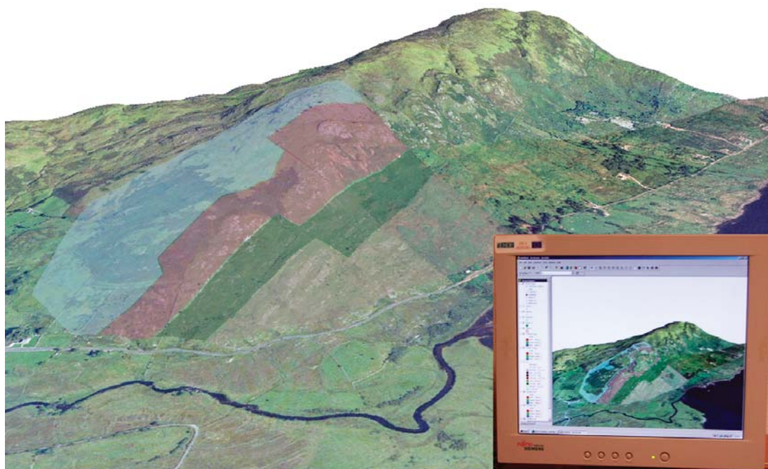
Figure 5. Student's geologic map of the Knock Kilbride field area, draped over a digital elevation model (DEM) of the mountain of Knock Kilbride (view to the northeast). By using a virtual 3-D model that incorporates high-resolution aerial photos, students can reevaluate their initial field interpretations to better constrain contacts and faults across the terrain.
