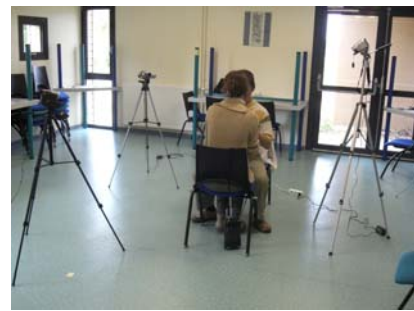
Figure 5: Optimal cameras position: one on each signer, one filming from above
